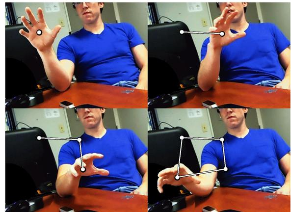
**Figure 1.** During calibration, the software guides users to position their hand at the 4 corners. Users can then rest their elbow on the table during the task, which reduces fatigue.
